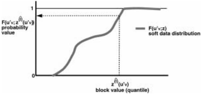
**Figure 2.** A schematic illustration showing how the probability value  $F(\mathbf{u}'_v; z^{(i)}(\mathbf{u}'_v))$  is taken directly from the soft data prior distribution given the local hard data average  $z^{(i)}(\mathbf{u}'_v)$ .
